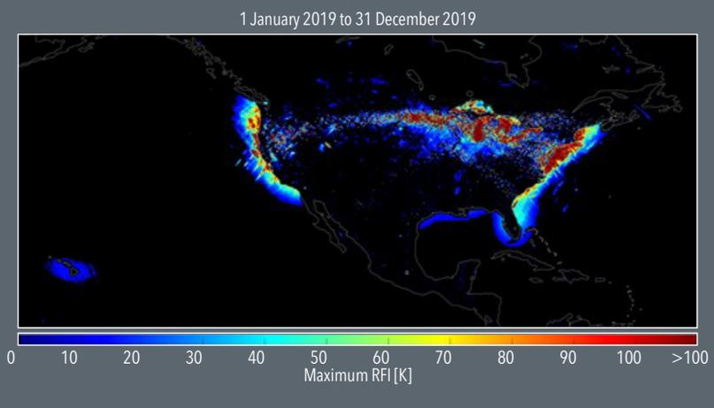
Figure 5 – Map of RFI power at C-band in Sentinel-1 Synthetic Aperture Radar measurements, with locations of weather radars superimposed.
